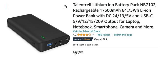
USB C can carry up to 5 amps however you need to verify that max current at each voltage you select on the battery. USB A is only good for 1.25 amps. However this batter is almost 10x a standard Baofend battery.
